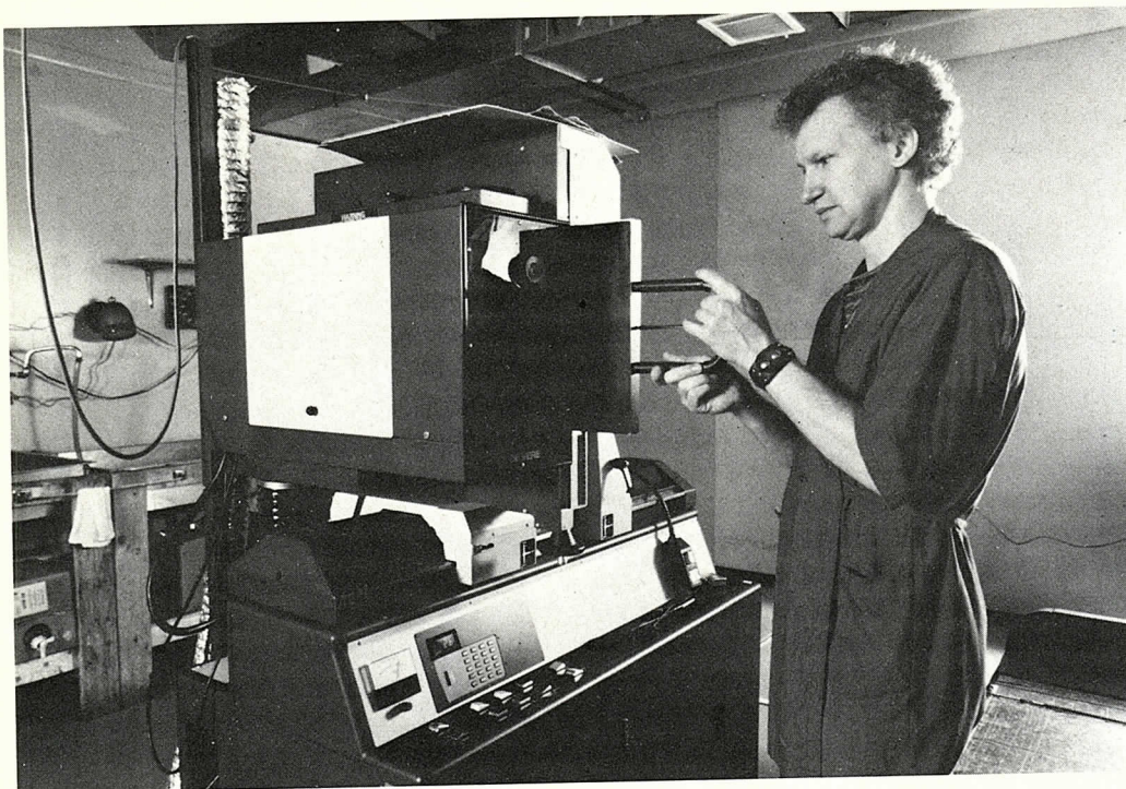
With over ten years of experience, mural printer Roger Bishop is a one-man operation. Using this vertical enlarger, a huge processor and dryer, he can produce b&w and colour sections of wall mural up to 48"x96".
