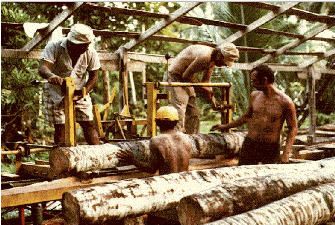
Rope driven, circular blade portable sawmill
